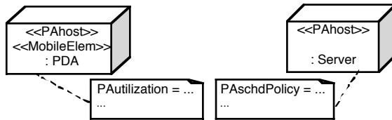
Fig. 19. Performance annotations for computing nodes in a UML-PMS model of a mobile system
