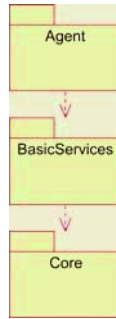
Fig. 7. 3-Layered Architecture of Hermes Mobile Computing Platform. The core supports identification, communication, loading and security; BasicServices supports discovery, mobility, creation, communication and security; Agent supports User agents and Service agents
